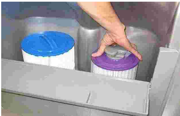
Figure 18. Screw-in Filter Removal
